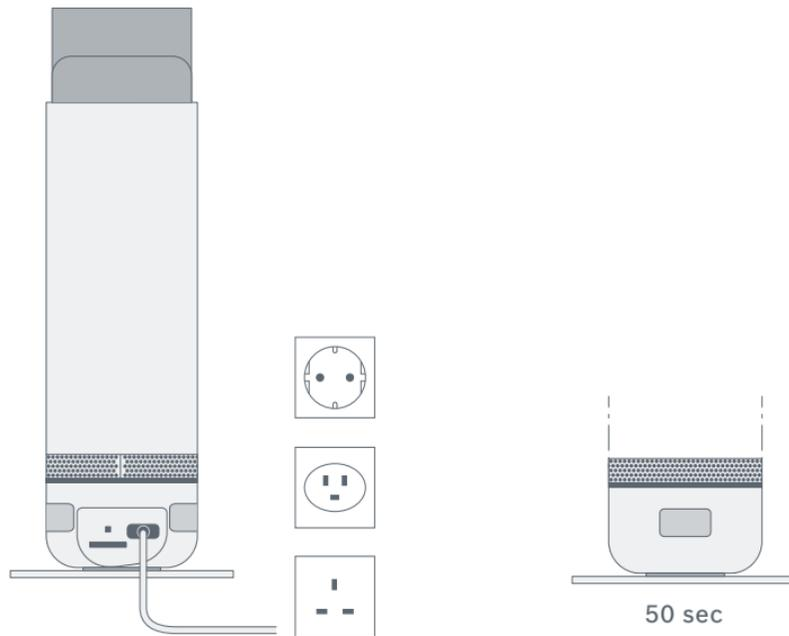
Connect the 360°-Indoor Camera via the power cable to the socket.
